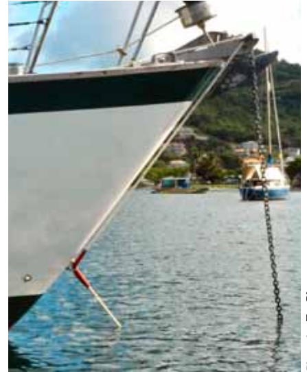
An eye-bolt on the stem of your boat allows you to lead a snubber line on to your anchor chain at a much lower angle
